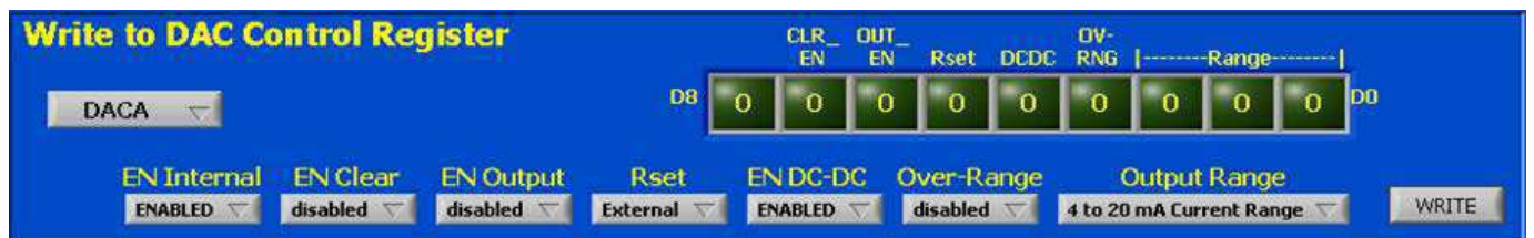
Figure 12. Write to the DAC Control Registers in the Evaluation Software
