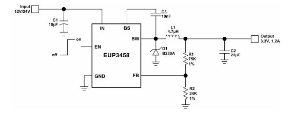
Figure 1. 12V/24V to 3.3V Application Circuit
