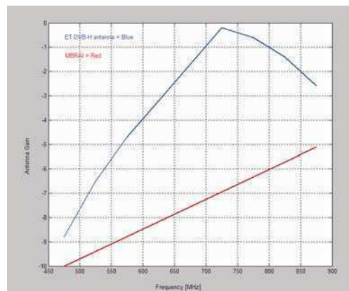
Ethertronics' UHF antenna gain solution performance: measured DVB-H gain compared to MBRAI specification
