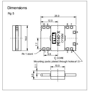
Dimensions shown are in millimetres. Terminal finish is 0.1µm max gold (Au) over nickel (Ni).
