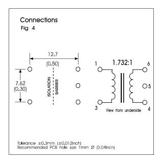
Dimensions shown are in millimetres (inches). Geometric centres of outline and pin grid coincide within a tolerance circle of 0.6mmØ.
