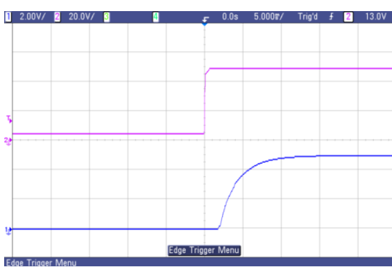
Fig.29 Typical start-up from power on of AVQ100B-48S05
