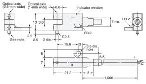
Vinyl-insulated round cable of 3.5 dia., 3 cores,
