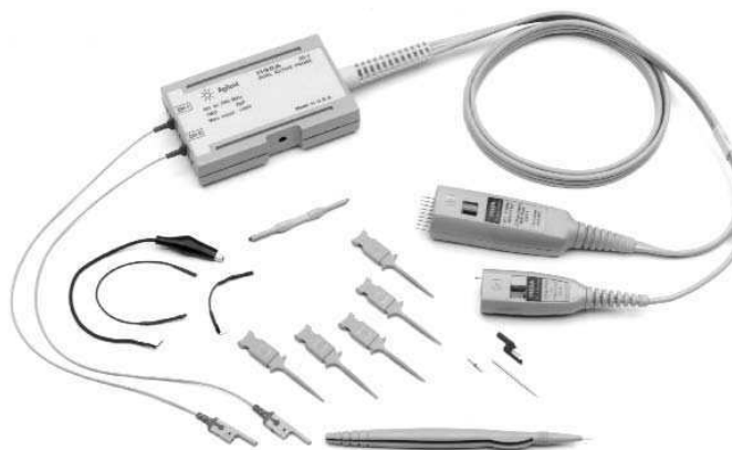
Figure 3.8. Agilent 1155A for fine-pitch ICs, SMDs, and dense circuit boards.
