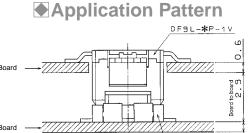
Note : The 2.9mm board to board size does not include the soldering paste thickness.
