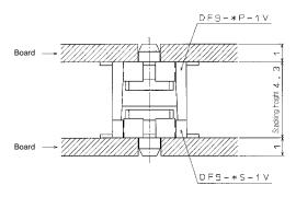
Note 1 : The board to board size 4.3mm in the pattern does not include the soldering paste thickness.
