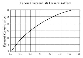
Forward Voltage VF(V)
