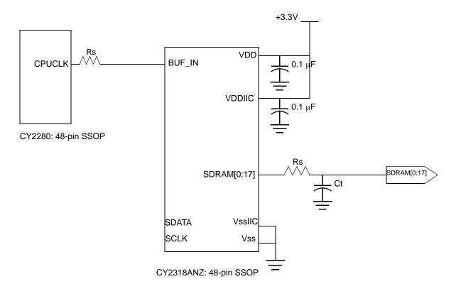
Rs = Series termination resistor Ct = Optional cap to reduce EMI
