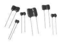
Ideal for snubber and RF applications, CDV16 mica capacitors now handle dV/dts up to 275,000 V/µs and they assure controlled, resonance-free performance through 1 GHz. CDV16/CD16 mica capacitors excel in both snubber applications and high-frequency applications like RF and CATV. Type CDV16's high pulse current capability make them ideal for pulse and snubber applications. CDV16 capacitors withstand an unlimited number of pulses with a dV/dt of 2 5,000 V/µs. This is a 20% increase in dV/dt
