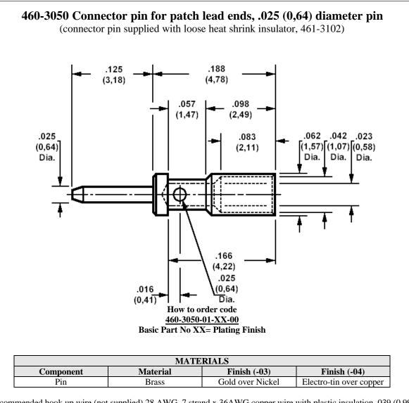
Recommended hook up wire (not supplied) 28 AWG, 7 strand x 36AWG copper wire with plastic insulation .039 (0,99) maximum diameter over insulation.
