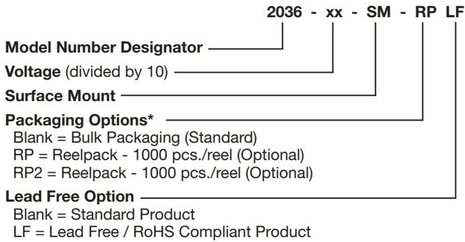
\* The optional -RP & -RP2 reelpacks contain 1000 pcs./reel. The reels are 330 mm in diameter. The -RP reelpack is 18 mm wide. The -RP2 reelpack is 26 mm wide.
