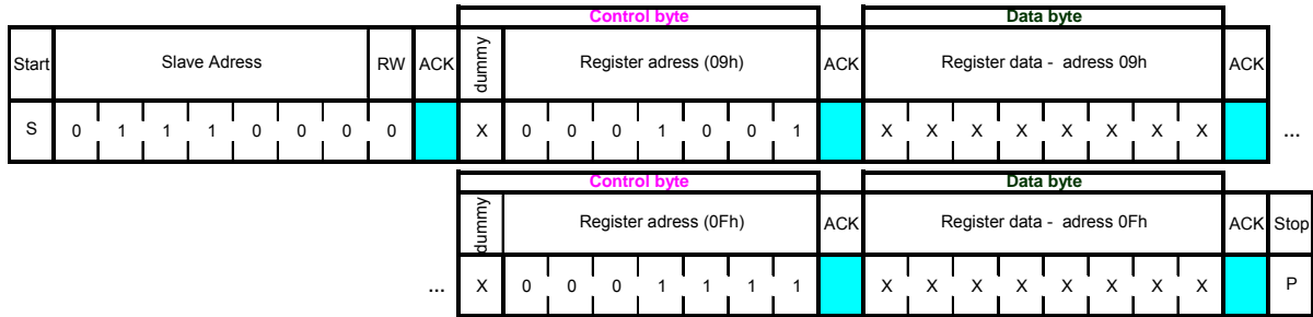
Figure 21: I 2 C multiple write protocol
