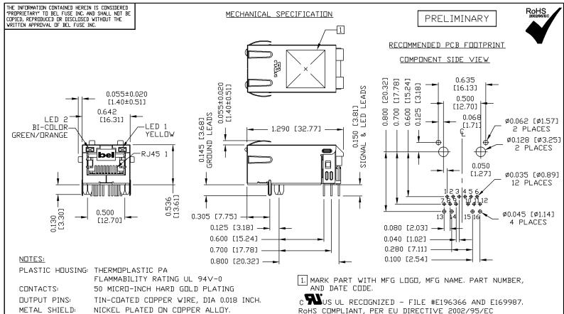
RoHS COMPLIANT, PER EU DIRECTIVE 2002/95/EC JACK CAVITY CONFORMS TO FCC RULES AND REGULATIONS.
