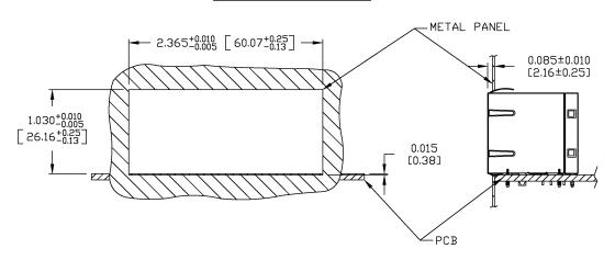
THE DISTANCE OF PANEL INSIDE SURFACE RELATIVE TO FRONT SURFACE OF PART IS ONLY A SUGGESTION. IN CASE THIS DISTANCE IS DIFFERENT, THE REQUIRED PANEL DANING DIMENSIONS CHANGE ACCORDINGLY.
