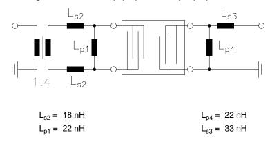
Element values depend upon PCB properties and layout. Transformer is only required for measurement in a  $50\Omega$  system.
