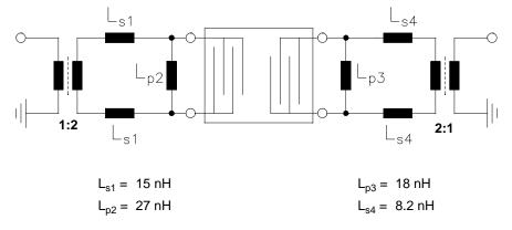
Element values depend upon PCB properties and layout. Transformers are only required for measurement in a  $50\Omega$  system.
