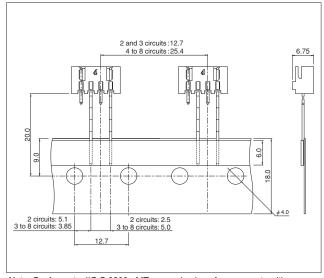
Note: Conforms to JIC C 0806 of "Tape packaging of components with unidirectional leads on continuous tapes".
