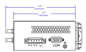
NOTE: These drawings reference the 716FX2 The 716FX2-HV dimensions are identical
