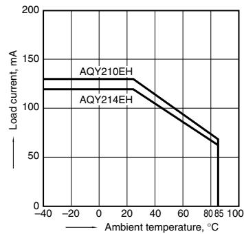
1-(2). Load current vs. ambient temperature characteristics
