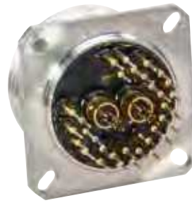
MIL-DTL-38999, SERIES III CONNECTOR WITH PC TAIL CONTACTS. This arrangement has 33 size 22D and 2 Quadrax PC tail contacts.
