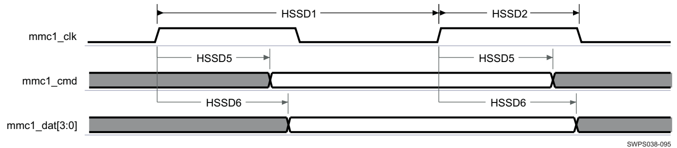
Figure 6-66. MMC1 Interface—High-Speed SD Mode—Data/Command Transmit
