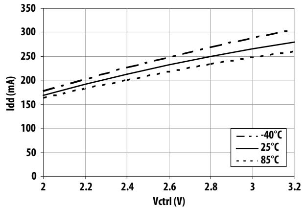
Figure 8. Idd vs. Vctrl and Temperature
