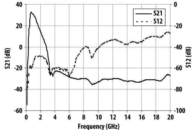
Figure 20.  $S_{21}$  &  $S_{12}$  vs. Frequency (0.1 to 20GHz)
