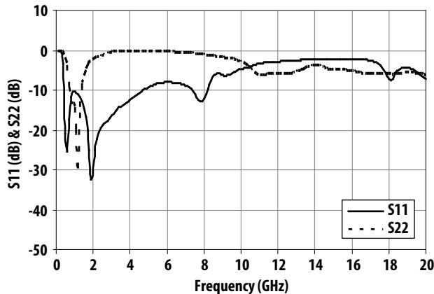
Figure 19.  $S_{11}$  &  $S_{22}$  vs. Frequency (0.1 to 20GHz)
