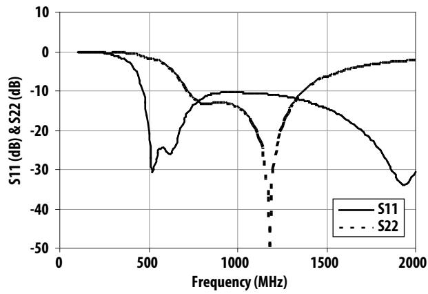
Figure 17. S11 & S22 vs. Frequency (0.1 to 2GHz)
