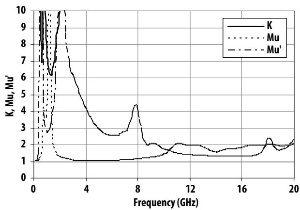
Figure 21. Stability vs. Frequency (0.1 to 20GHz)
