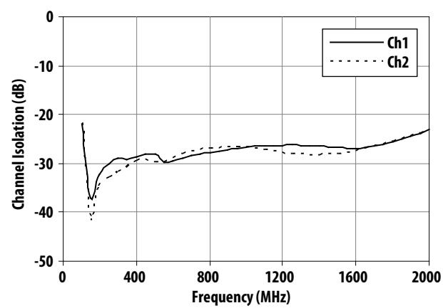
Figure 22. Channel Isolation vs. Frequency (0.1 to 2GHz)
