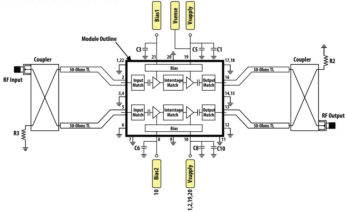
Figure 24. Evaluation Board Schematic for Balanced Amplifier
