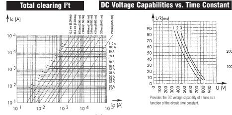
Above: Horizontal curves show maximum values of total clearing I2t (I2tt) as function of prospective current lp. @  $U_{\mbox{\scriptsize N}}$  with  $\cos j = 0.15$  Oblique lines indicatye total clearing duration Tt and associated pre-arching duration in brackets.
