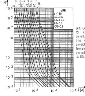
Left: Curves show, each rated for current, pre-arching time vs. R.M.S. pre-arching current. Tolerance for mean pre-arching current
