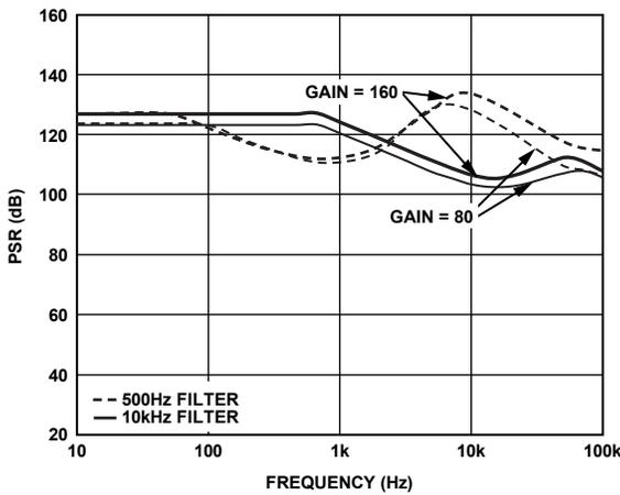
Figure 12. Power Supply Rejection (PSR) vs. Frequency
