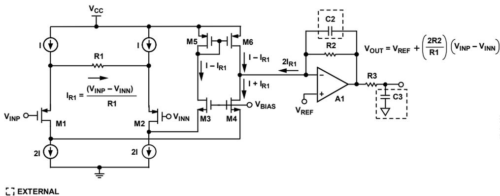
Figure 18. Simplified Schematic
