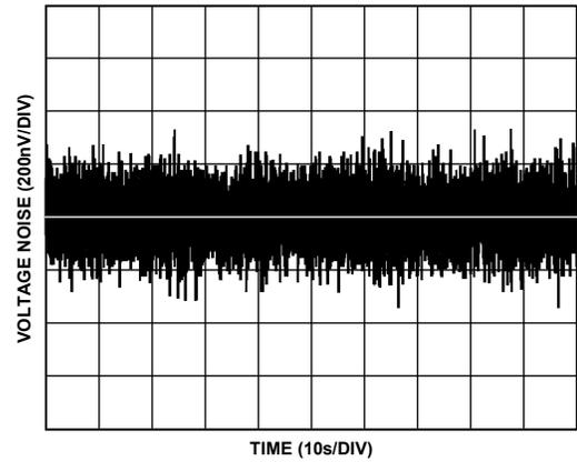
Figure 14. 0.01 Hz to 10 Hz Voltage Noise
