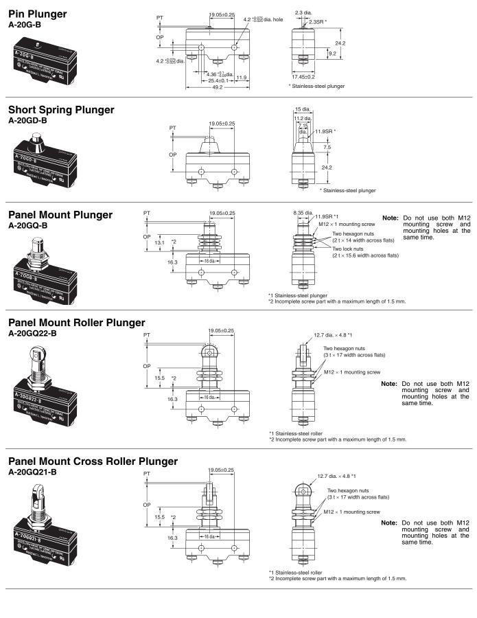
**Note: 1.** All drawings show the switches with screw terminals. For solder terminals, remove the "-B" from the end of the part number **2.** Unless otherwise specified, all units are in millimeters and a tolerance of  $\pm$  0.4 mm applies to all dimensions.
