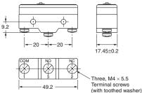
Note: Appropriate terminal screw tightening torque: 0.78 to 1.18 N·m.
