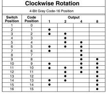
Indicates closed circuit; blank indicates open circuit.
