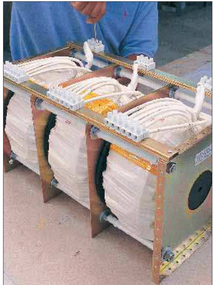
3-Phase Toroidal Array Mounted in Flanges with Terminal Blocks
