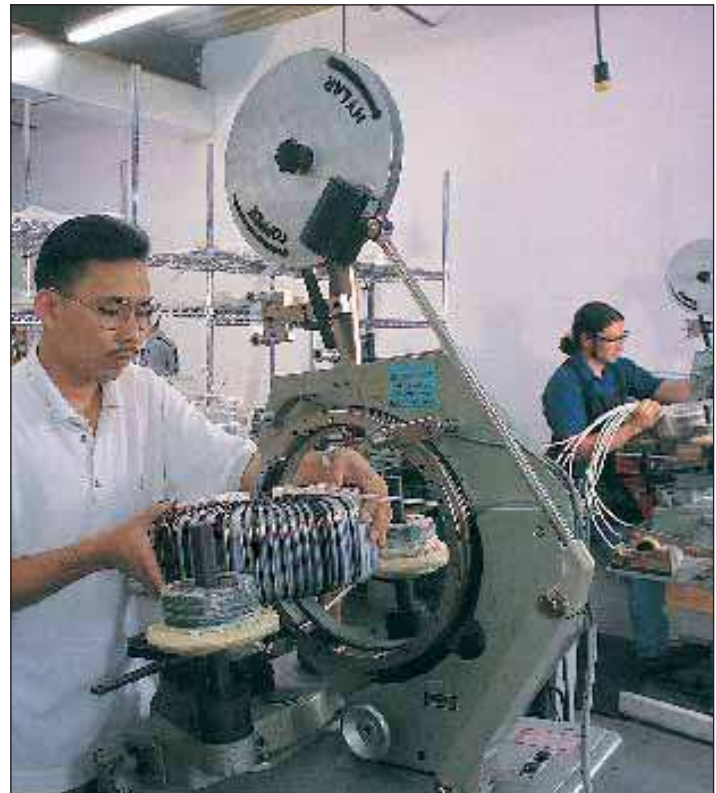
Applying Part of the Insulation System
