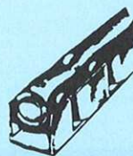
2. Insulation being pierced.
