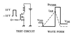
$$\begin{aligned} &R_G = 25~\Omega \\ &V_{DD} = 90~V,~L = 12~mH \end{aligned} \qquad E_{AS} = \frac{1}{2} \cdot L \cdot I^2 \cdot \left(\frac{B_{VDSS}}{B_{VDSS} - V_{DD}}\right) \end{aligned}$$
