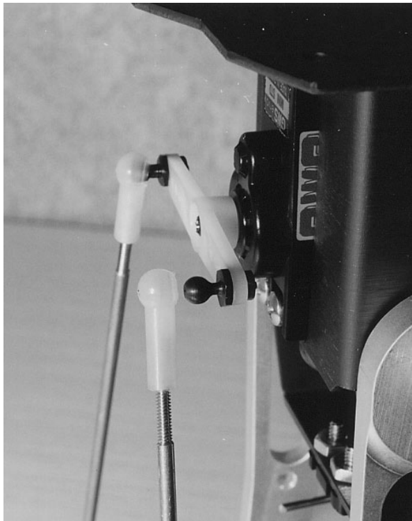
Figure 1-17 Install tilt rods.
