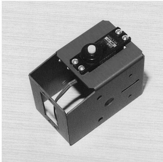
Figure 1-1 Install Tilt Servo in Body
