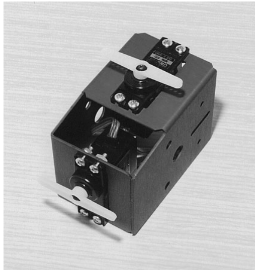
Figure 1-4 Both servo horns are installed on centered servos.
