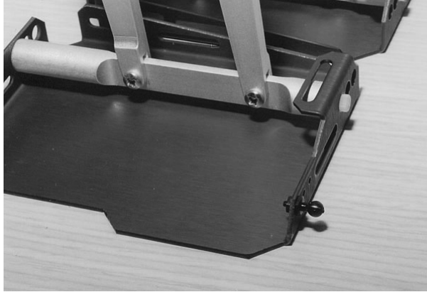
Figure 1-15 Install ball joints on feet.
