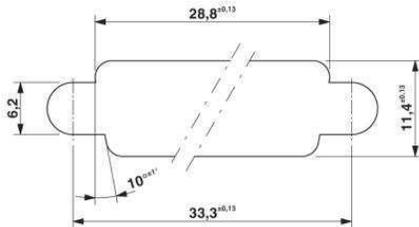
Panel cutout in acc. with DIN 41652-3 for wall up to 4.5 mm thick
