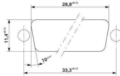
Panel cutout in acc. with DIN 41652-3 for wall up to 2.0 mm thick
