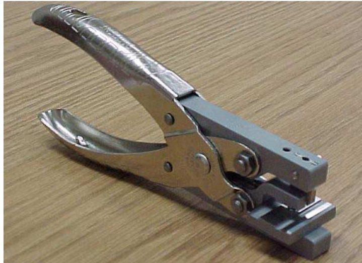
Figure 24 BPY75D37 Wire Insertion Repair Tool
