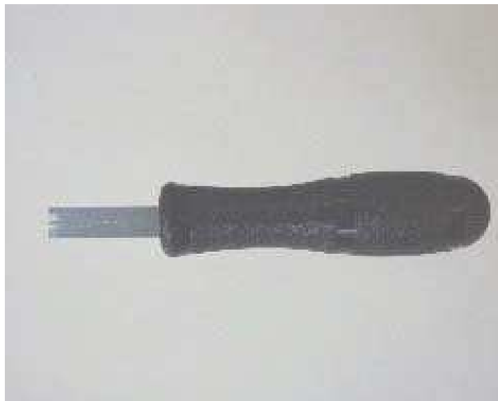
Figure 24 BPY75D37 Wire Insertion Repair Tool
