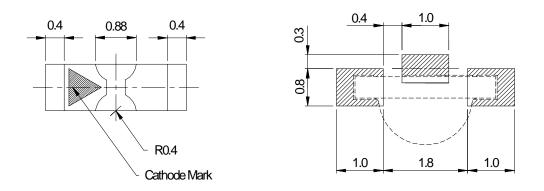
**Note:** The tolerances unless mentioned is  $\pm 0.05$  mm, Unit = mm
