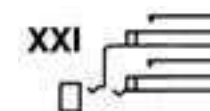
Double open circuit. Isolated switching—separate "make" circuits on both tip and ring. (J2-2A).
