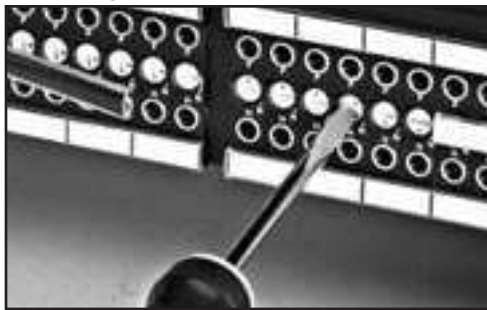
Center Strip Removes For Normaling Access
