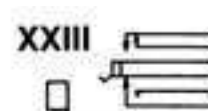
Single closed circuit plus "make" before "break". Isolated switching—"make" before "break" circuit. (J8-1D).
