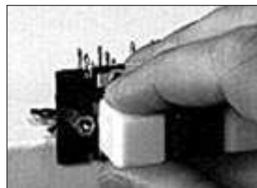
Squeeze upper and lower surfaces of pushbutton and pull free of plungers.
